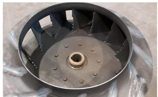
Figure 5: Manually Pre-Damaged Impeller.
